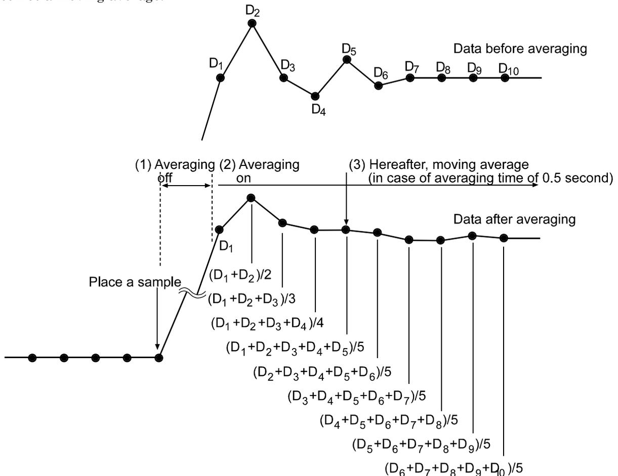
For very small samples or when filling very small amounts, fluctuations in the display can be small (not exceeding averaging range set by “Averaging range”) and the averaging process may not turn off. If the averaging process does not turn off when a sample is added, the balance will stay in the moving averaging state, and it will take longer to reach the final value after the sample is placed on the balance.
