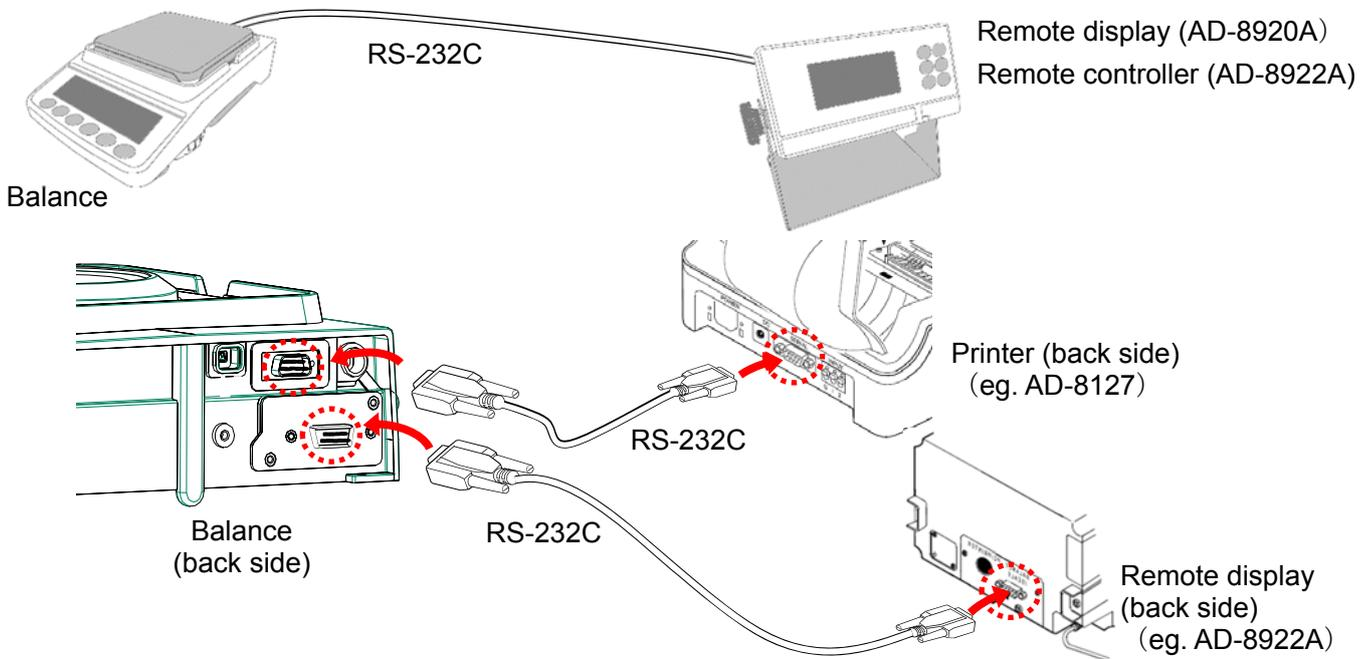
It is also possible to connect a printer to a remote controller (AD-8922A). For details, please refer to the AD-8922A instruction manual.
