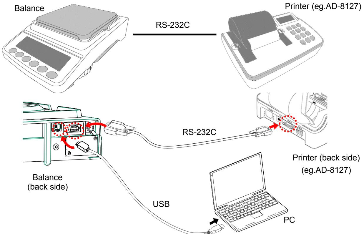
If only the balance is connected to the PC, it can also be connected using a USB cable or RS-232C cable.
