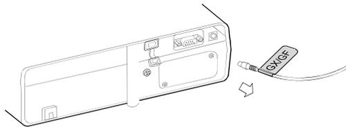
2. Connect the balance and the PC via a USB cable.
