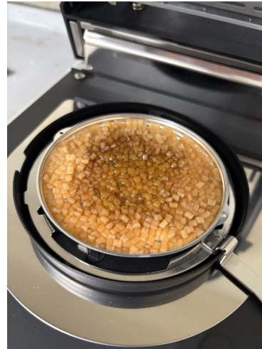
Higher than appropriate drying temperature setting
