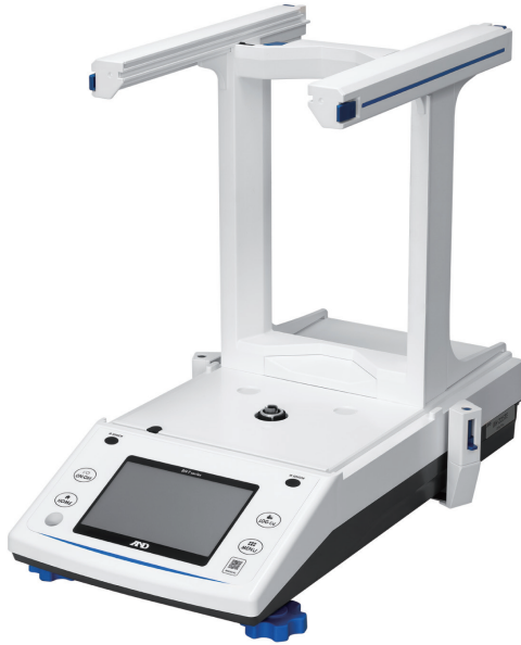
Glass panes and floor plate fully removed
